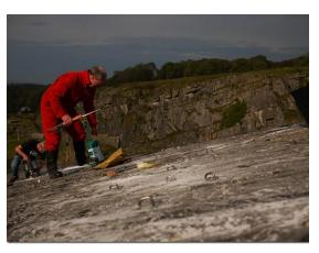
secured in the substrate using Allgrip KMR-RES chemical anchor mortar which is a polyester resin with styrene. The anchors were left unloaded for 1 day until test to failure on 24<sup>th</sup> September 2011.
